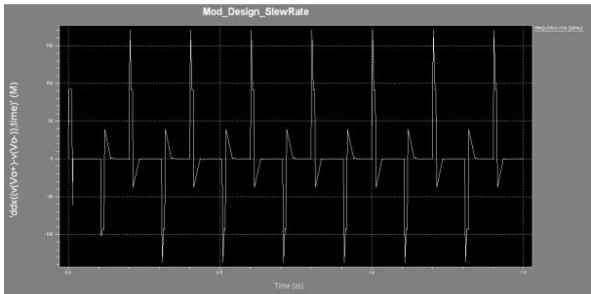
Fig 9: Slew rate for proposed telescopic Op-Amp
